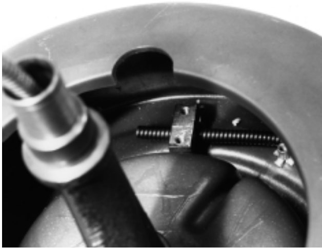
Figure 16 – Position New Cable Under Bracket
