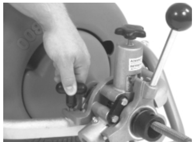
Figure 4 – Mounting the Autofeed Onto the Frame
