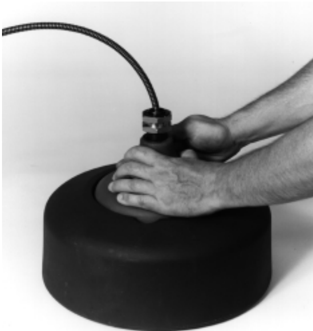
Figure 13 – Removing Cable End
