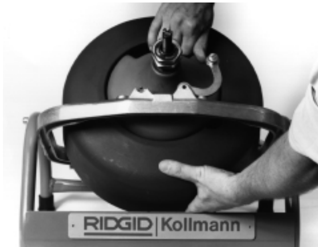
Figure 2 – Aligning Drum and Gearbox Bore
