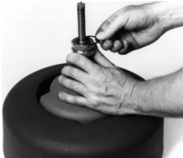
Figure 17 – Reassemble Inner Drum, Front Bracket and E-Clips
