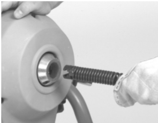
Figure 4 – Inserting Cable Into Front Of Machine
