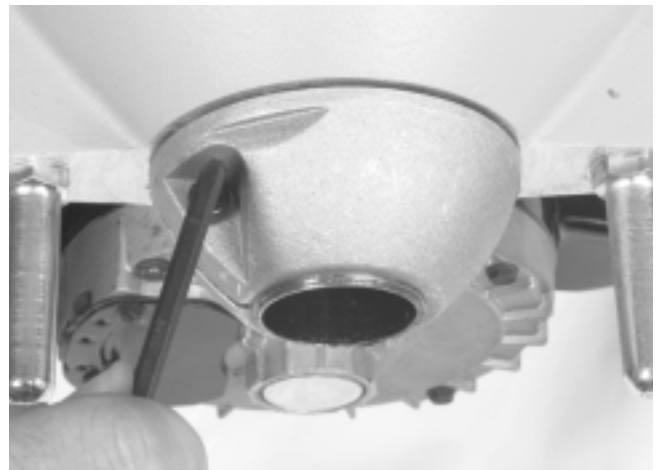
Figure 14 – Removing Clutch End Play
