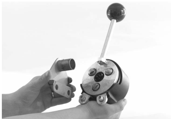
Figure 3 – Placing Mounting Bracket Into AUTOFEED
