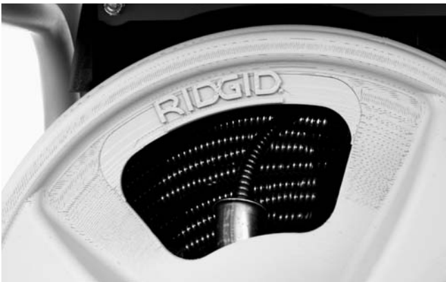
Figure 17 – Coil Cable Into Drum As Shown
