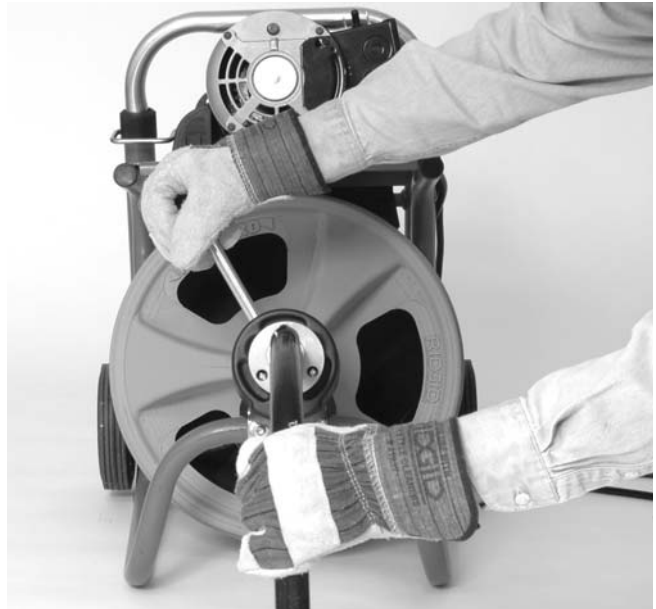
Figure 15 – Using Machine with Guide Hose
